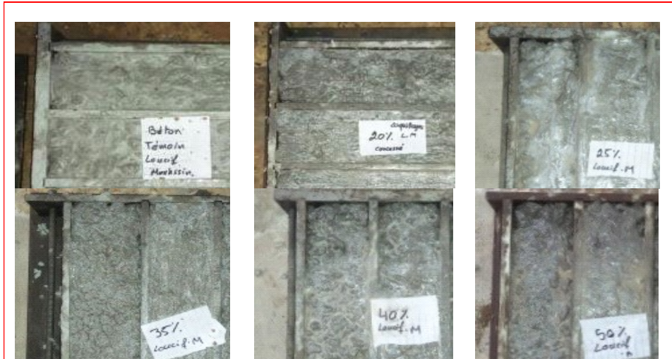
Fig. 3. Concrete poured into test tube molds
